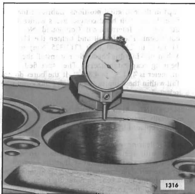
Fig. 5 - Checking Depth of Counterbore with Tool J 22273
