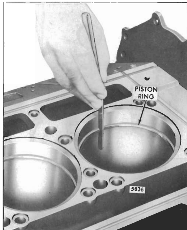
Fig. 14 - Measuring Piston Ring Gap
