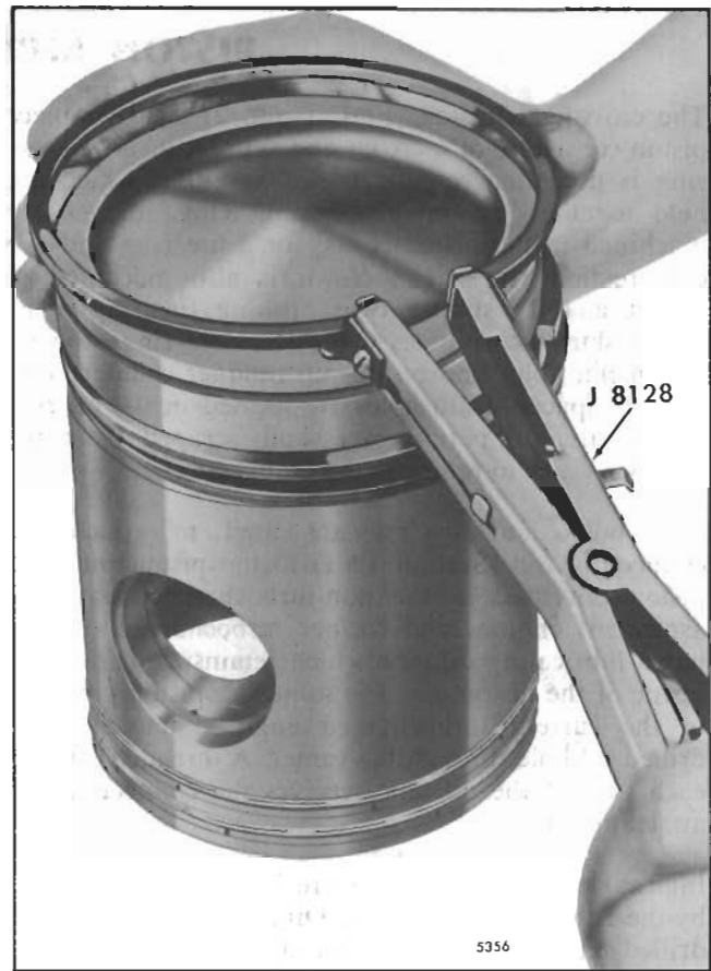
Fig. 4 - Removing or Installing Piston Rings
