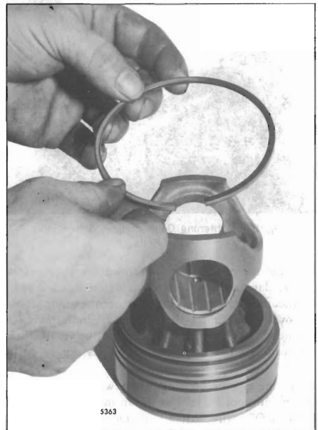
Fig. 6 - Installing Seal Ring
