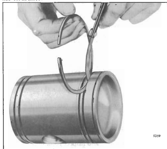
Fig. 15 - Measuring Piston Ring Side Clearance
