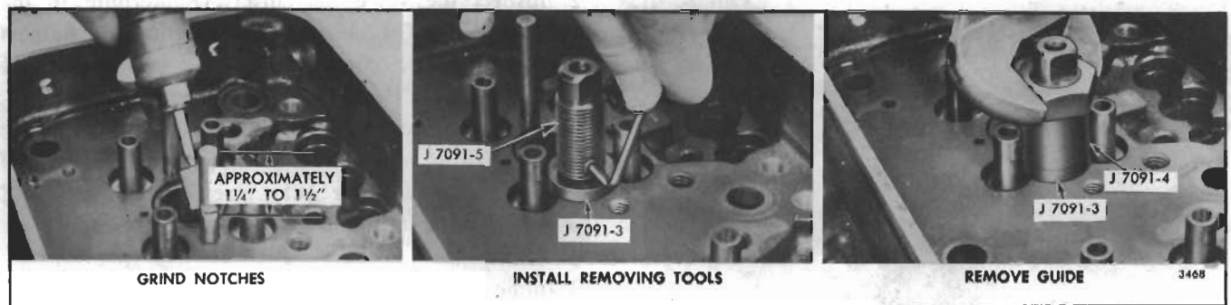
Fig. 8 - Removing Press-Fit Exhaust Valve Bridge Guide
