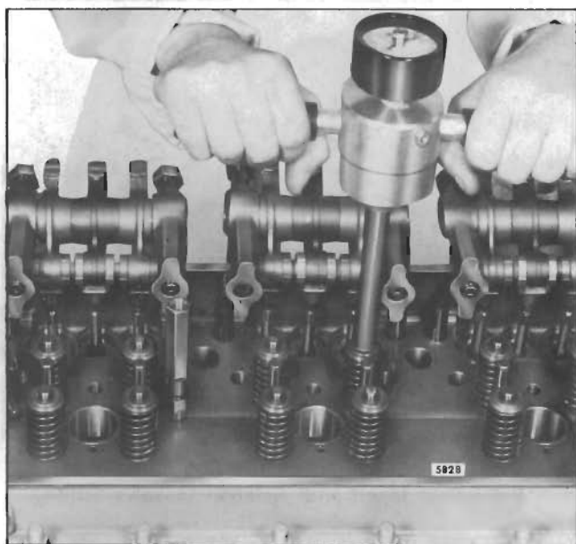
Fig. 15 - Checking Pressure Required to Open the Exhaust Valve in Cylinder Head
