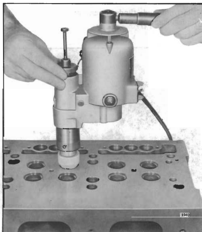
Fig. 12 - Grinding Valve Seat Insert
