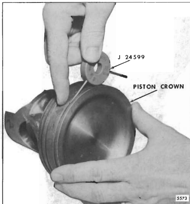
Fig. 5 - Checking Fire Ring Groove in Piston Crown
