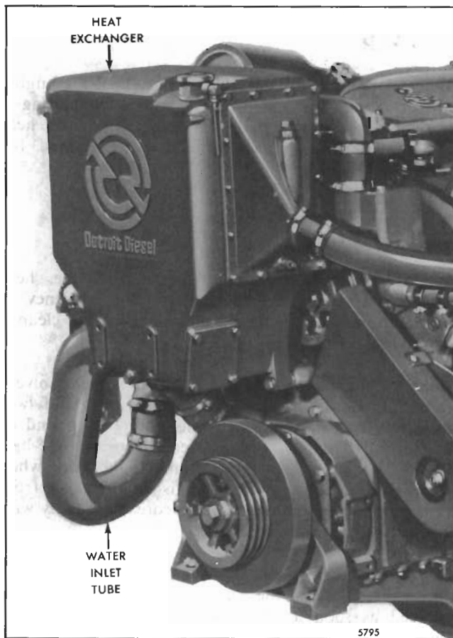
Fig. 1 - Typical Heat Exchanger Mounting
