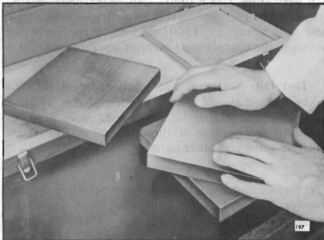
Fig. 2 - Refinishing Lapping Blocks
