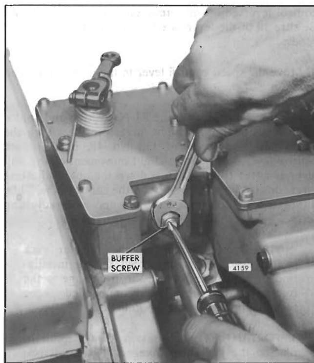
Fig. 8 - Adjusting Buffer Screw
